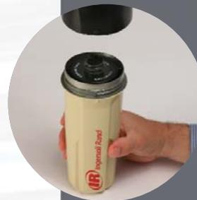
1. Turning the filter bowl counter-clockwise disengages the element from the filter head, allowing it to drop down into the bowl.
