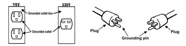
**5-2-5-1**: This product is for use on a nominal 115 or 230 volt circuit · A cord with a grounding plug as shown here shall be used · Make sure that the product is connected to an outlet having the same configuration as the plug · No adapter should be used with this product ·
