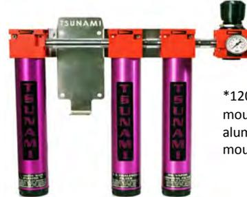
\*120SCFM packages mounted with heavy duty aluminum extrusion mounts
