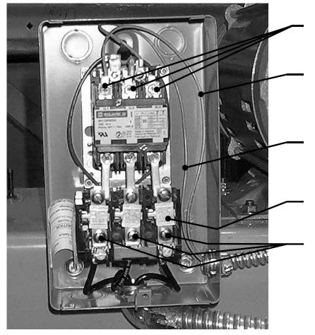
CONNECT INCOMING POWER WIRES TO STARTER TERMINALS L1, L2, L3
