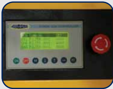
PLC Controller monitors maintenance, temp, oil level, filtration, hours, plus remote start/stop
