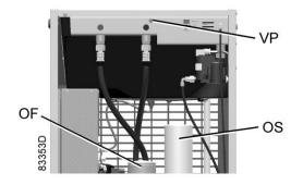
Vent plug, oil cooler Workplace
