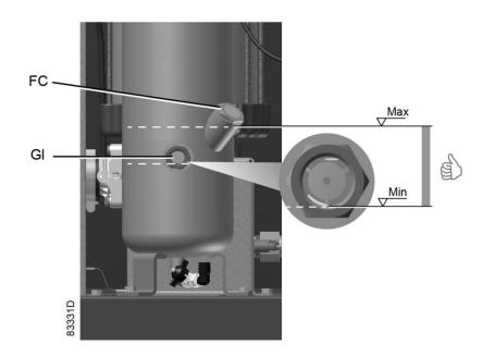
A few minutes after stopping, the oil level should reach the bottom of the oil filler neck (FC).
