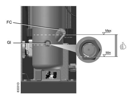
Take care that no dirt drops into the system. Refit and tighten filler plug (FC).
