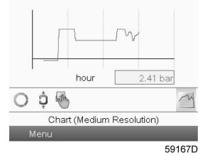
When the Chart (Medium Resolution) is selected, the chart shows the variation of the selected input <u>per</u> <u>hour</u>. The screen shows the last 4 hours.
