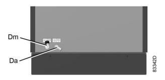
Condensate drain connections, typical example
