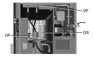
Vent plug, oil cooler Workplace Full-Feature
