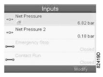
The first item in the list is highlighted. In this example, the Net Pressure is selected (chart icon). To change, press the Enter button again: a pop-up window opens:
