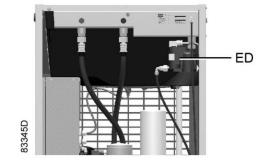
Location of electronic water drain (Workplace)
