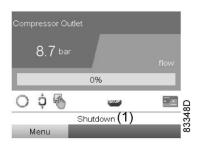
Typical display when the compressor is stopped by a shutdown
