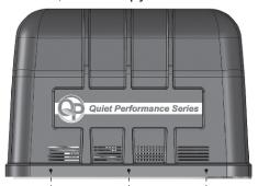
To remove the canopy, simply remove the 6 fasteners and lift the canopy straight up and off.
