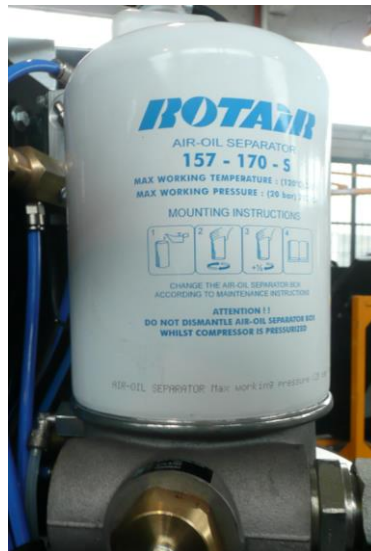
Figure 13.4-7 Oil separator filter
