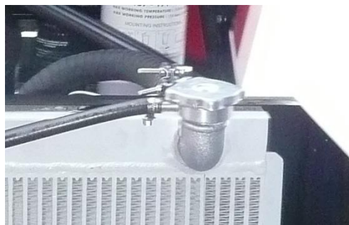
Figure 10.1-3 Checking the radiator cooling liquid
