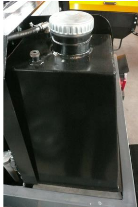
Figure 10.1-2 Fuel tank for Diesel engine
