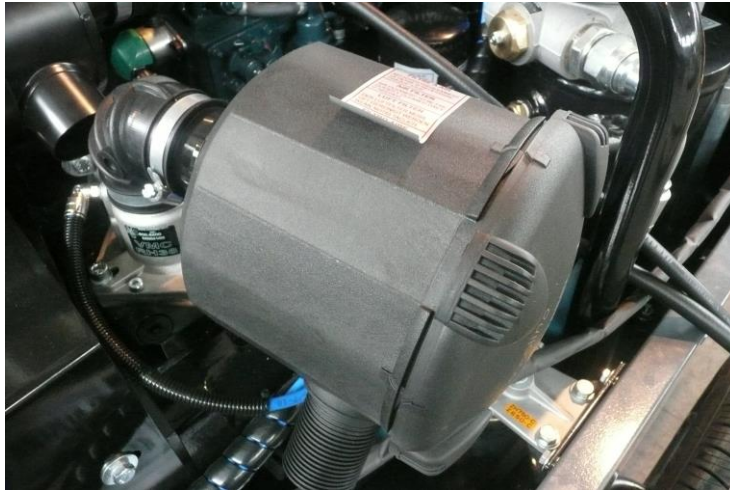
Figure 13.4-1 Aspiration air filter
