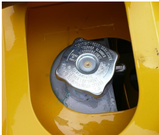
Figure 10.1-3 Checking the radiator cooling liquid
