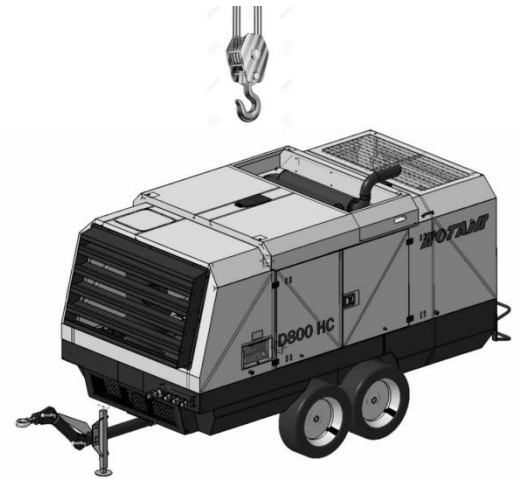
Figure 6.2-1 Lifting system of the machinery
