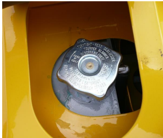
Figure 12.4-3 Checking the coolant radiator
