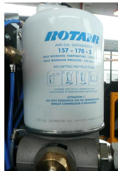
Figure 13.4-7 Oil separator filter
