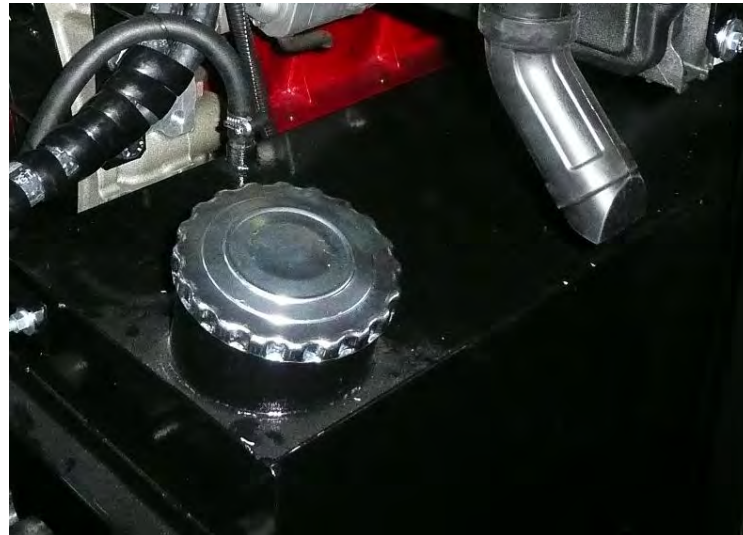
Figure 10.1-2 Gas oil tank for Diesel engine
