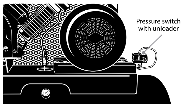
Figure 2: Install unloader line from check valve to pressure switch
