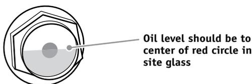
**Figure 3: Check proper oil level**
