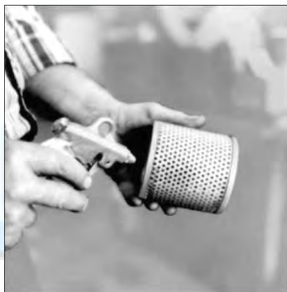
Cleaning the air filter
