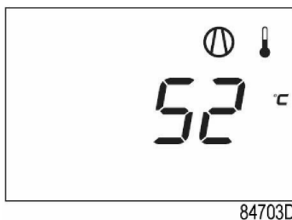
Main screen with temperature (stopped compressor)
