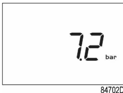
Main screen with pressure (stopped compressor)
