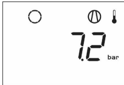
84711D Main screen with shutdown indication, element outlet temperature
