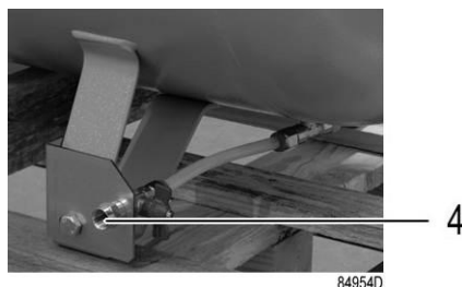
Condensate drain valve on air receiver
