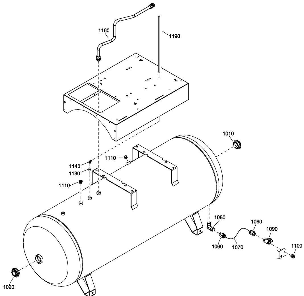
**13 - Air Outlet Pack - Tank mounted - 500L**
