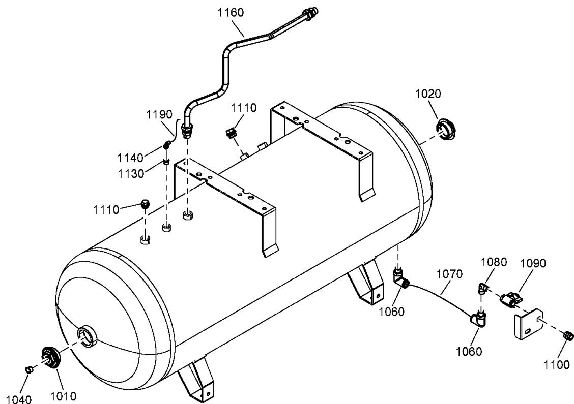
**12 - Air Outlet Pack - Tank mounted - 270L**
