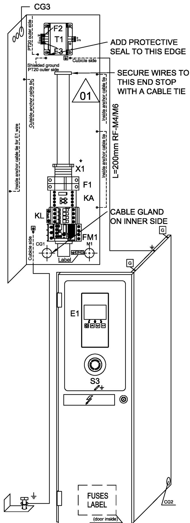
**36 - Cubicle components QGS 15 - 575V/60Hz - UL-cUL**
