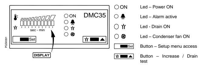
The DMC35 displays DewPoint temperature, controls the condenser fan activation, controls the timed drainer and keep record of the total hours of operation of the dryer.
