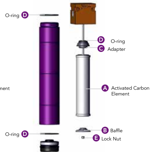
Figure 5 : Activated Carbon Filter
