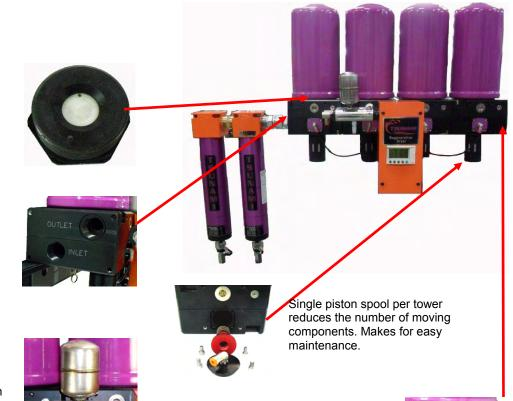
Dryer housings are machined from solid aluminum billet. Hard coat anodize provides superior strength and corrosion
